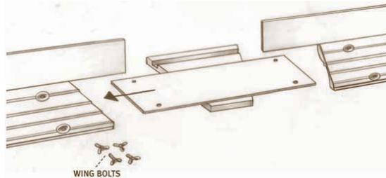
Turn both sides of the cornice and the keystone over onto their FACE and lay on a flat surface. Slide the keystone onto one side of the cornice as shown above. When assembled, the dustcover top of the cornice should be in the channel in the back of the keystone and the bolt holes in the keystone and in the back of the cornice should align.
